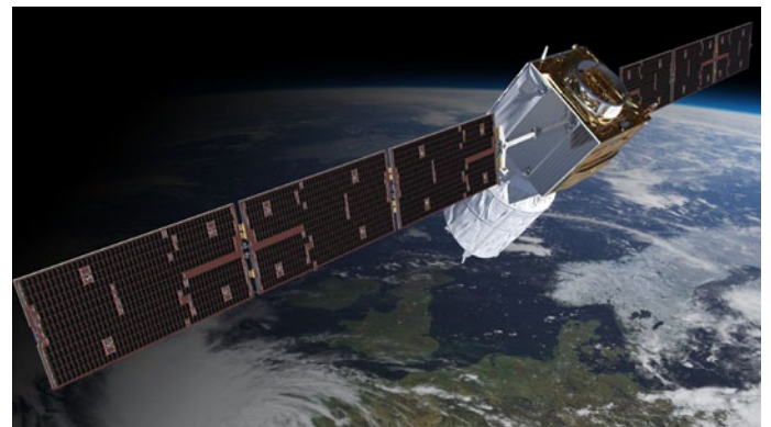
ADM-Aeolus is the first space mission to acquire profiles of the wind on a global scale. These near-realtime observations will improve the accuracy of numerical weather and climate prediction and advance our understanding of tropical dynamics and processes relevant to climate variability. Picture © ESA.
